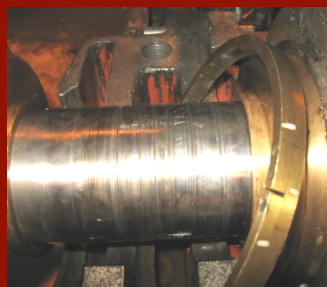
Scored seal journals on a Boiler feed pump is repaired in situ with only the removal of the seal and bearing housing
