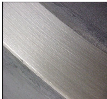
Damages are filled with nickel and finished to the original size and tolerance.
