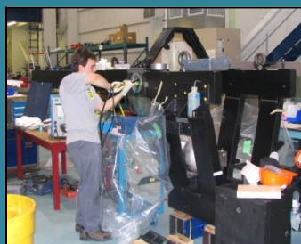
Brush Plating repair done on an oversized bearing fit on an FM Frame unit.
