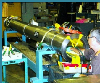
Score damage on I.D. of the RAM barrel housing being repaired with Brush Nickel Plating.
