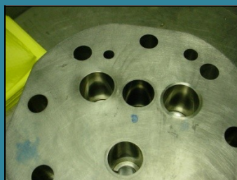
CMC's Brush Plating technique for repair of separator bores - maintaining a very tight .0002" tolerance.
