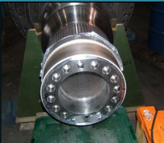
A worn 24" undersized bearing journal is built to size in place without the need of grinding.
