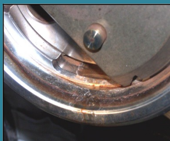
Deep pitting and corrosion damage (.025" deep) caused major refueling problems.
