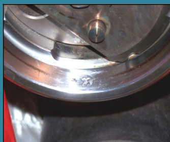
During an outage, Brush Plating repair was completed in 3 hours at the reactor face.
